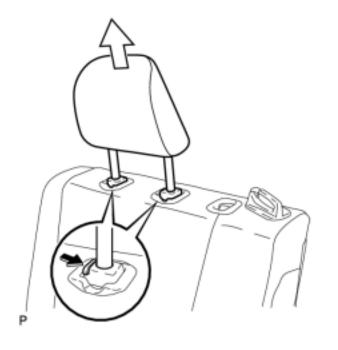
(a) Press the 2 headrest support buttons and pull up the rear seat headrest assembly LH as shown in the illustration.
