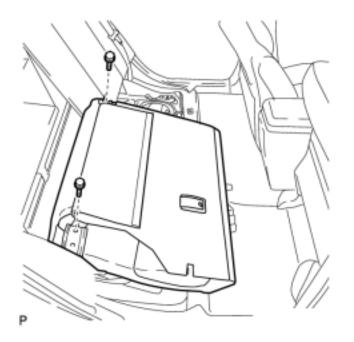
(c) Remove the 2 bolts and rear seatback assembly RH.
