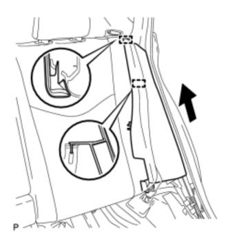
(b) Disengage the 2 guides and remove the rear side seatback assembly LH as shown in the illustration.
