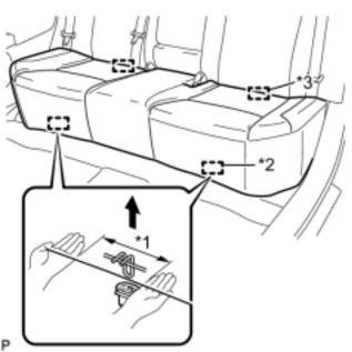
(a) Disengage the 2 front hooks of the seat cushion from the vehicle body as shown in the illustration.
