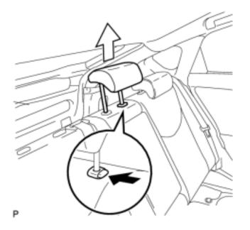
(a) Press the headrest support button and pull up the rear seat center headrest assembly as shown in the illustration.
