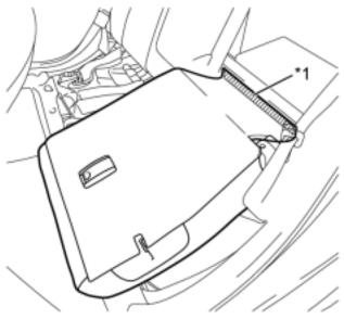
(b) Disengage the fastener.
