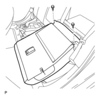
(c) Remove the 2 bolts and rear seatback assembly LH.
