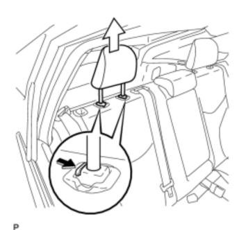
(a) Press the 2 headrest support buttons and pull up the rear seat headrest assembly RH as shown in the illustration.
