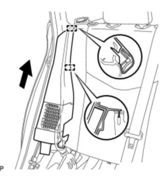
(b) Disengage the 2 guides and remove the rear side seatback assembly RH as shown in the illustration.
