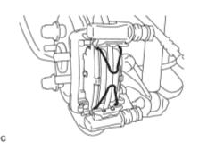
(a) Remove the 2 anti-squeal springs from the rear disc brake pads.
