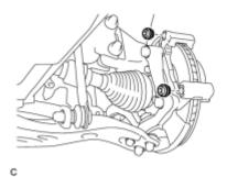
(b) Install the 2 front disc brake bushing dust boots to the front disc brake cylinder mounting.
