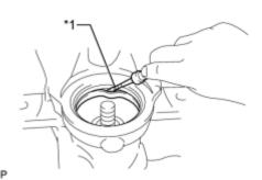
(a) Using a screwdriver with its tip wrapped with vinyl tape, remove the piston seal from the rear disc brake cylinder assembly.
