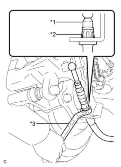
(b) Separate the No. 3 parking brake cable assembly from the rear disc brake cylinder assembly.
