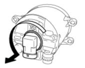
(a) Turn the fog light bulb in the direction indicated by the arrow shown in the illustration and remove it.
