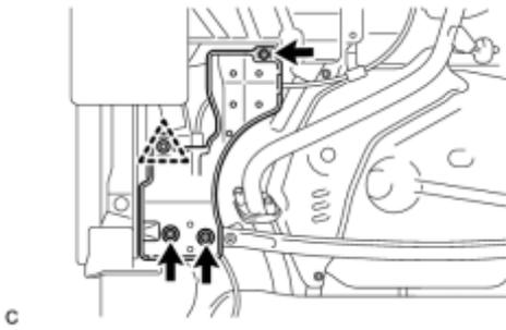
(b) Install the rear floor side member cover RH with the 3 bolts.
