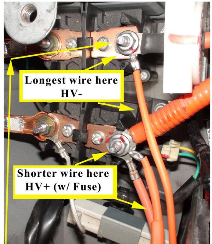
Remove the 8mm bolts on top of the relay and install the wires as shown. The wire with the fuse goes on the rear relay.
