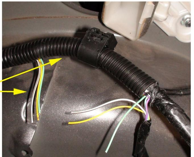
Install the fan board as shown (left photo). The wires are installed from closest to farthest from the fan: White w/ Black, Yellow, {empty}, Green. Clean the wheel well location where the fan board will mount using glass cleaner or similar. Secure the fan board to the vehicle using the tape affixed on the back, firmly pressing it into place.
