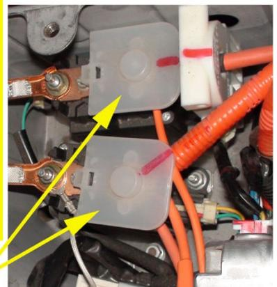
Route the orange HV leads as shown. The shorter wire with the fuse is the **HV+**, the longer wire is the **HV-**.
