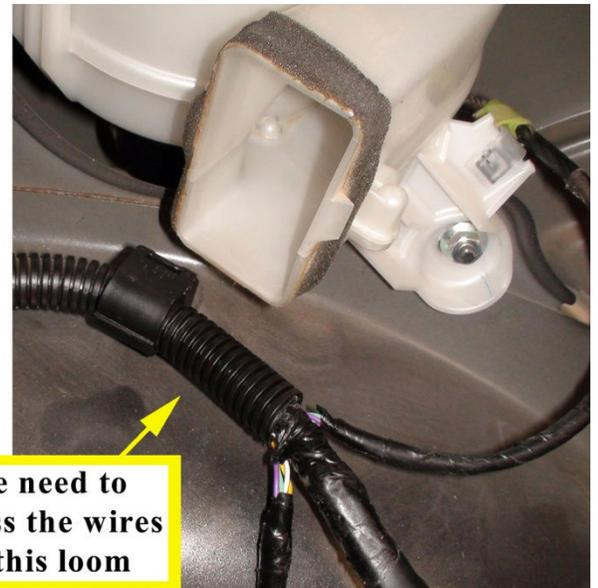
Unclip the loom and open the bracket holding the loom. Remove the tape and slide the loom off of the wires as shown. Isolate and cut the three wires (White w/ Black strip, Yellow, Green). Reassemble the loom, leaving the three cut wires accessible. Reattach the clip and secure it back in place on its bracket. Strip ¼" off of each end of the 3 exposed wires.
