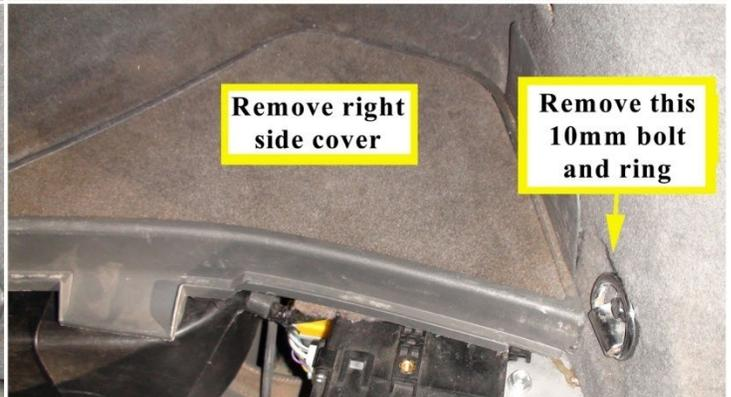
Next we will remove the cover over the battery. This is held in place by two 10mm bolts (removed in previous step) and 3 plastic clips. Velcro attaches the carpet in the front of the cover to the rear seat backs. Pull up on the cover to detach the 3 clips and remove the cover.
