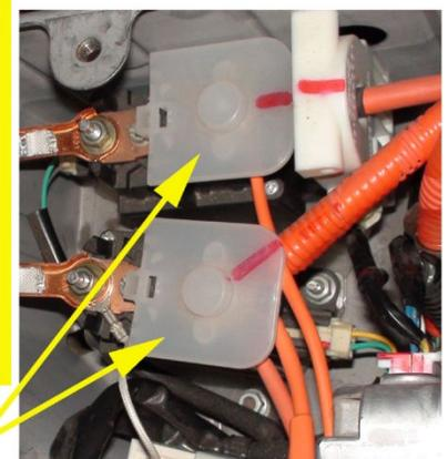
Route the orange HV leads as shown. The shorter wire with the fuse is the **HV+**, the longer wire is the **HV-**.
