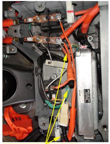
Route the orange HV leads as shown. The shorter wire with the fuse is the HV+, the longer wire is the HV-.
