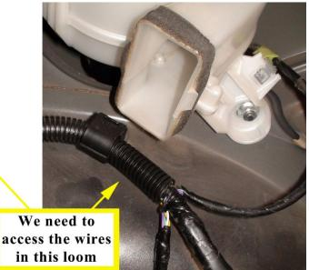
Unclip the loom and open the bracket holding the loom. Remove the tape and slide the loom off of the wires as shown. Isolate and cut the three wires (White w/ Black strip, Yellow, Green). Reassemble the loom, leaving the three cut wires accessible. Reattach the clip and secure it back in place on its bracket. Strip  $\frac{1}{4}$ " off of each end of the 3 exposed wires.
