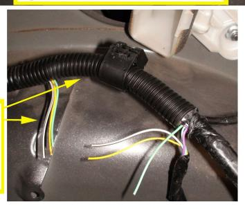
Install the fan board as shown (left photo). The wires are installed from closest to farthest from the fan: White w/ Black, Yellow, {*empty*}, Green. Clean the wheel well location where the fan board will mount using glass cleaner or similar. Secure the fan board to the vehicle using the tape affixed on the back, firmly pressing it into place.
