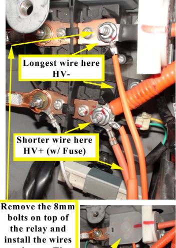
install the wires as shown. The wire with the fuse goes on the rear relay.
