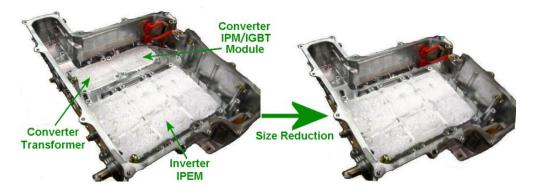
Fig. 5.15. Conceptual change to inverter/converter casing for excluding the buck/boost converter.
