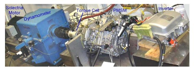
Fig. 3.16. The test hardware for Prius performance characterization tests.
