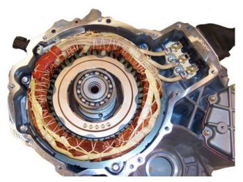
Fig. 2.8. 2004 Prius motor rotor and stator.
