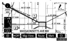
The current vehicle position mark ( $\boxed{1}$ ) appears in the center or bottom center of the map screen.
