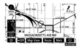
When your vehicle is receiving signals from the satellites, the "GPS" mark appears at the top left of the screen.
