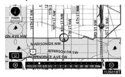
Touch or to change the scale of the map display. The scale bar and indicator at the bottom of the screen indicates the map scale menu. The scale range is 150 feet (50 m) to 250 miles (400 km).
