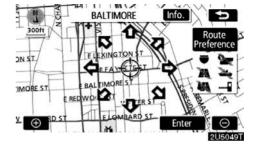
1. When an arrow facing the desired point is touched, the map scrolls in that direction.
