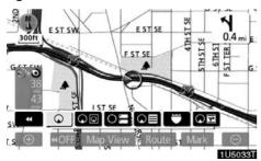
2. To select the desired screen configuration, touch one of the following buttons. Depending on the conditions, certain screen configuration buttons cannot be selected.
