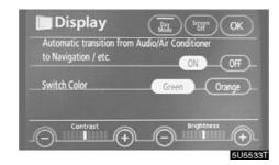
Depending on the position of the headlight switch, the screen changes to the day mode or night mode.
