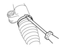
(a) Using a screwdriver, remove the No. 2 steering rack boot clamp.
