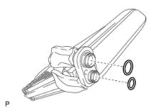
(e) Remove the 2 O-rings from the cooler evaporator sub-assembly.
