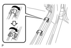
(a) Disengage each claw to open the 2 door scuff plate clamps as shown in the illustration.
