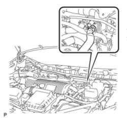
(a) Using pliers, grip the claws of the clip and slide the clip to disconnect the outlet heater water hose.
