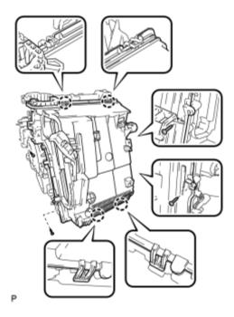
(e) Install the lower heater case with the 4 screws.
