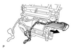
(c) Remove the quick heater assembly as shown in the illustration.
