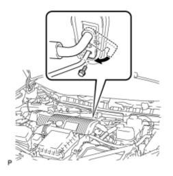
(e) Move the hook connector in the direction indicated by the arrow in the illustration.
