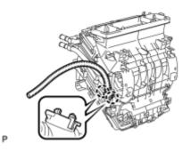
(a) Disengage the 2 claws and remove the air conditioning duct subassembly.
