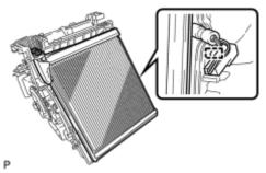
(c) Engage the clamp and install the cooler evaporator sub-assembly with the No. 1 cooler thermistor.
