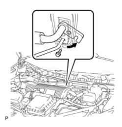
(a) Remove the bolt and slide the hook connector.
