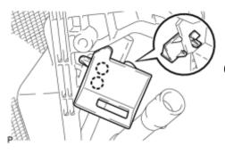
(a) Engage the 2 claws and install the console mounting bracket RH.
