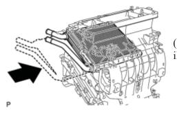
(a) Install the heater radiator unit sub-assembly as shown in the illustration.
