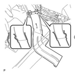
(a) Engage the 2 claws to install the rear No. 2 air duct.
