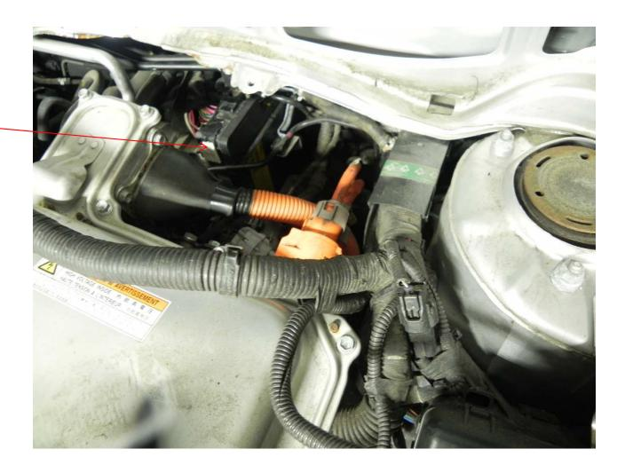
View of connector on Actuator Perform resistance measurements to check if actuator has failed. See next slide.
