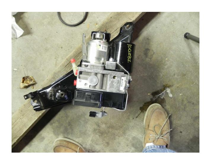
Remove damper from bracket, and remove bracket, replace actuator for reassembly. Follow directions in reverse to reassemble.
