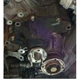
Old, leaking water pump
