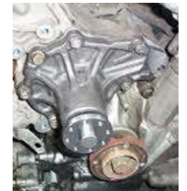
New water pump
