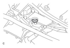
(b) Using a hexagon wrench (10 mm), remove the drain plug indicated in the illustration and drain the coolant.
