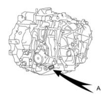
(b) The transaxle code is stamped on the case as shown in the illustration.
