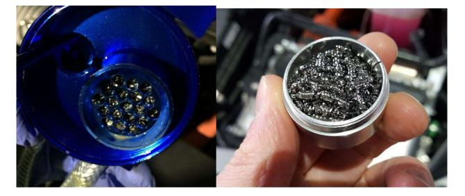
Make sure that filtering material what you use cannot get to exhaust of the OCC and to the intake manifold.
