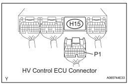
(a) Disconnect the H15 HV control ECU connector.
