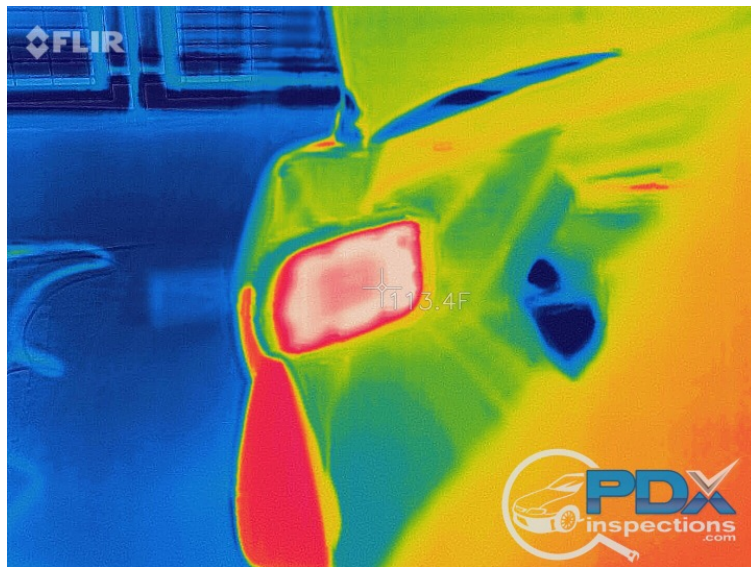
Heated mirror operation verified with an infrared camera
