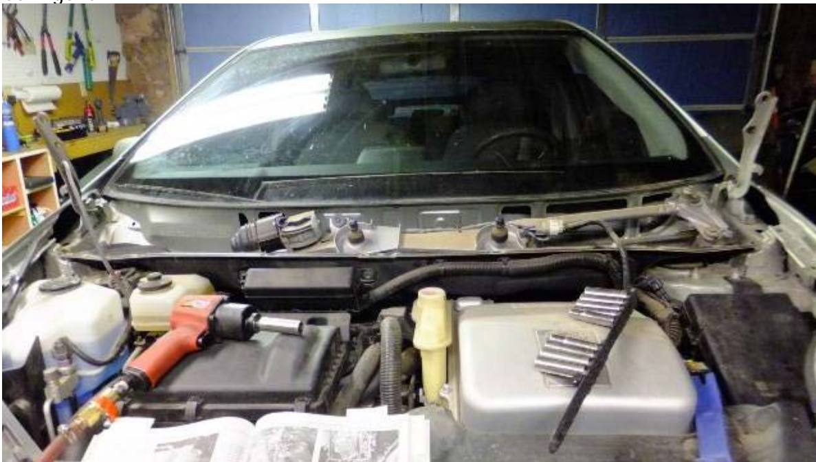
19) Unbolt the 5 10mm bolts holding down the wiper motor assembly and remove.
