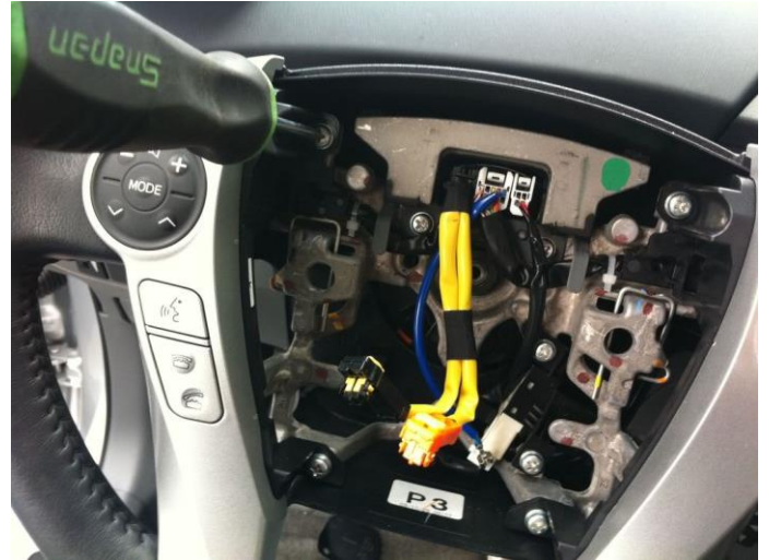
The instrument cover is also held on by 4 screws, 2 on each side top and bottom remove those two and pull the cover out.
