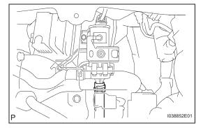
(b) Slide the hose clip and then disconnect the heater water hose C.
