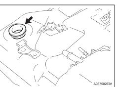
(e) Remove the gasket from the fuel tank.
