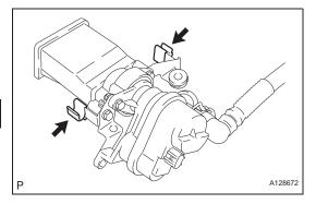
(c) Install the 2 clamps to the trap canister with pump module.
