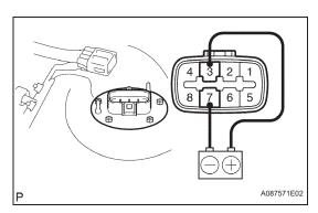
(b) Check that the motor operates when battery voltage is applied across the terminals.
