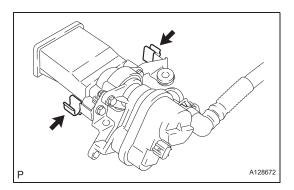
(f) Remove the 2 clamps from the trap canister with pump module.
