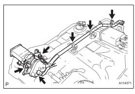
(d) Install the trap canister with pump module and connect the ground terminal of the fuel tank wire with the 2 bolts.
