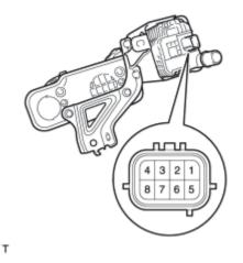
(1) Connect a positive (+) lead of the battery to terminal 5 and a negative (-) lead to terminal 1.
