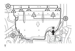
(b) Install the rear floor step under cover sub-assembly with the nut and 5 clips (A).
