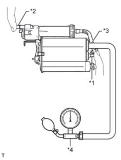
(1) Connect a pressure gauge to the vent port of the charcoal canister.
