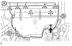
(a) Remove the 5 clips (A) and nut.
