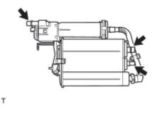
(1) Visually check the charcoal canister for cracks or damage.
