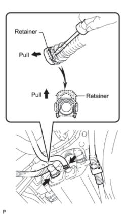
(b) Disconnect the tube clamp, purge line hose and vent line tube.
