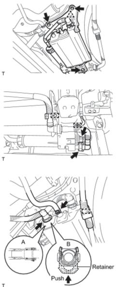
(a) Install the charcoal canister assembly with the 3 bolts and clip.
