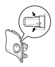
(a) Attach the 2 claws to install the power switch.
