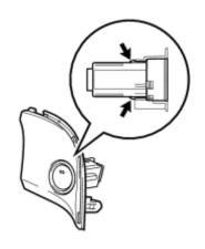
(a) Detach the 2 claws and remove the power switch.
