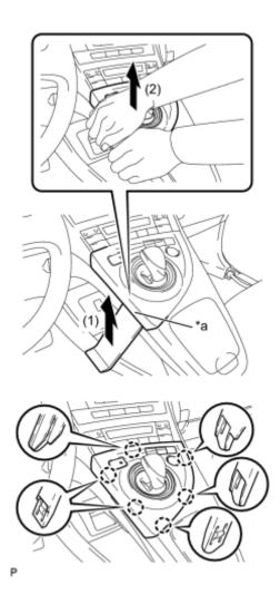
(b) Pull the integration control and panel assembly in the direction indicated by the arrow to disengage the 6 claws.
