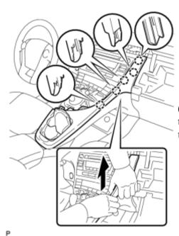
(b) Pull the lower center instrument cluster finish panel sub-assembly in the direction indicated by the arrow to disengage the 5 claws and remove the lower center instrument cluster finish panel sub-assembly.
