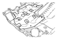
(a) Using hot-melt glue and install a new No. 2 instrument panel cushion as shown in the illustration.
