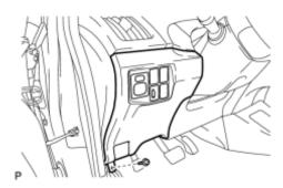
(e) Install the lower instrument panel finish panel assembly with the screw <*C*>.
