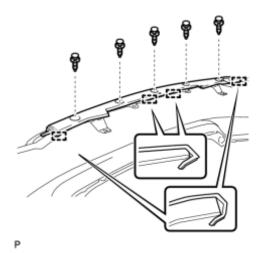
(b) Disengage the 4 guides and remove the rear No. 1 spoiler.
