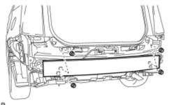
(a) Install the No. 1 rear bumper reinforcement with the 4 nuts.
