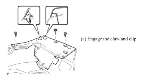
(b) Install the rear side spoiler sub-assembly RH with the 3 screws.
