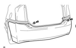
(e) Engage the 2 rear bumper upper stoppers and install the 2 screws.
