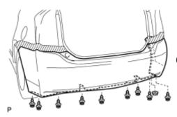
(c) Using a clip remover, remove the 9 clips.
