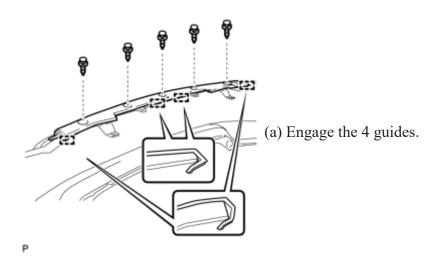
(b) Install the rear No. 1 spoiler with the 5 clips.
