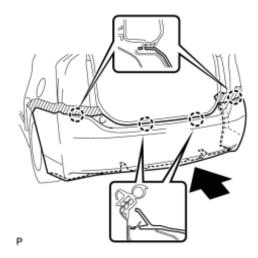
(a) Engage the 4 claws and install the rear bumper assembly as shown in the illustration.
