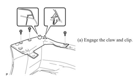
(b) Install the rear side spoiler sub-assembly LH with the 3 screws.
