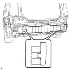
(a) Engage the 2 guides to install the rear bumper energy absorber.
