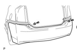
(b) Remove the 2 screws and 2 rear bumper upper stoppers.
