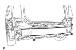
(a) Remove the 4 nuts and No. 1 rear bumper reinforcement.
