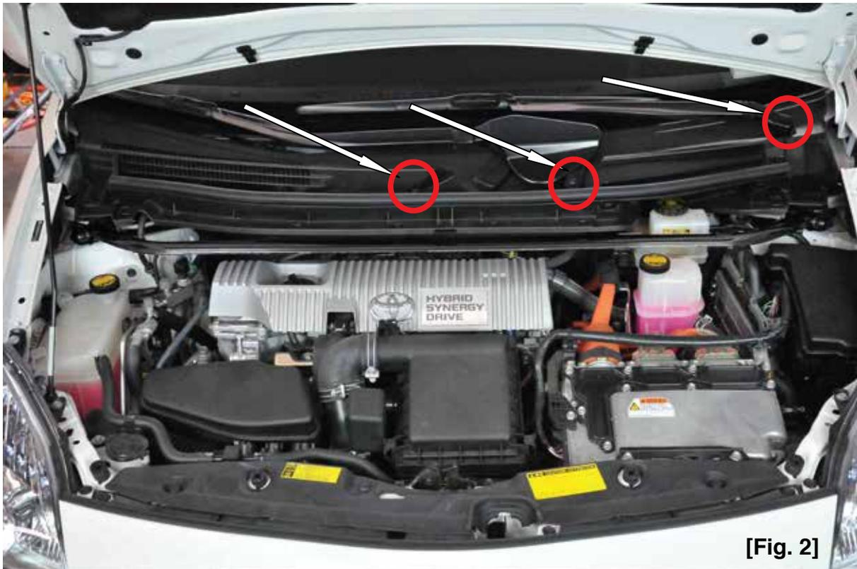
3.) Remove two plastic clips located on the left and right corners of the plastic cowl. Pop in the center dowel first to easily pull off the clip.
