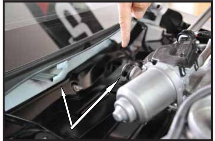
6.) Remove three 10mm bolts to take off the bracket located in the center (Fig. 4) followed by nine 10mm bolts (Fig. 5) to completely take off the large metal shielding pan.
