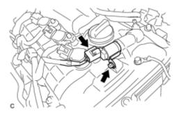
(b) Install the camshaft timing oil control valve assembly and wire harness bracket with the bolt.
