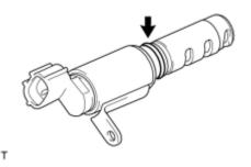
(c) Remove the O-ring from the camshaft timing oil control valve assembly.
