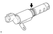
(a) Apply a light coat of engine oil to a new O-ring and install it onto the camshaft timing oil control valve assembly.
