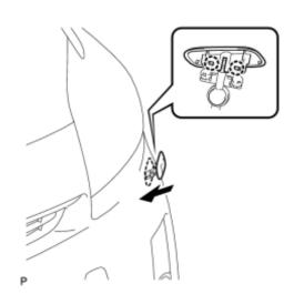
(a) Engage the 2 claws to install the headlight cleaner washer nozzle.
