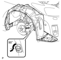
(a) Using a screwdriver, turn the pin 90 degrees and remove the pin hold clip.
