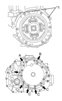
(b) Using an engine lifter, align the engine assembly and hybrid vehicle transaxle assembly, fit the knock pins into the knock pin holes, and tighten the 7 bolts shown in the illustration.
