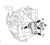
(a) Install the rear engine mounting bracket with the 4 bolts in several steps.
