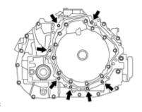
(b) Remove the 7 bolts and hybrid vehicle transaxle assembly.
