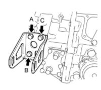
(a) Install the front engine mounting bracket with the 3 bolts in several steps.
