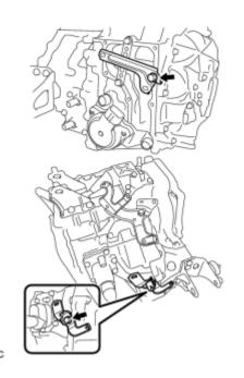
(a) Install the 2 wire harness clamp brackets with the 2 bolts.
