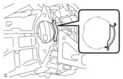
(a) Remove the flywheel housing side cover.
