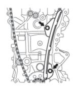
(a) Remove the 2 bolts and chain vibration damper.
