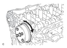
(f) Turn the camshaft timing gear within its movable range (26.5 to 28.5°) 2 or 3 times without turning it to the most retarded position. Make sure that the camshaft timing gear turns smoothly.
