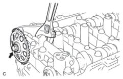
(a) Remove the flange bolt while holding the hexagonal portion of the camshaft with a wrench, and then remove the camshaft timing sprocket.
