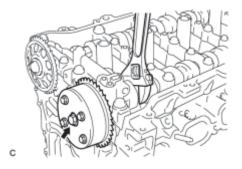
(d) Tighten the flange bolt with the camshaft timing gear secured in place.
