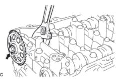
(a) Tighten the flange bolt with the camshaft timing sprocket secured in place.
