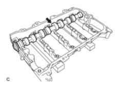
(c) Install the No. 2 camshaft to the camshaft housing.
