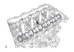
(a) Remove the camshaft.
