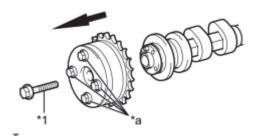
• Keep the camshaft timing gear horizontal while removing it from the camshaft.
