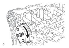
(e) Check that the camshaft timing gear can move in the retard direction (clockwise) and is locked in the most retarded position.
