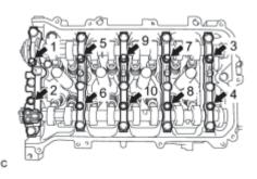
(a) Uniformly loosen and remove the 10 bearing cap bolts in the sequence shown in the illustration.
