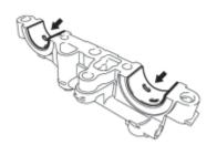
(a) Remove the 2 No. 1 camshaft bearings.
