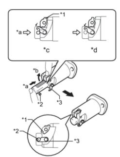
(a) Release the cam, and then fully push in the plunger and engage the hook to the pin so that the plunger is in the position shown in the illustration.
