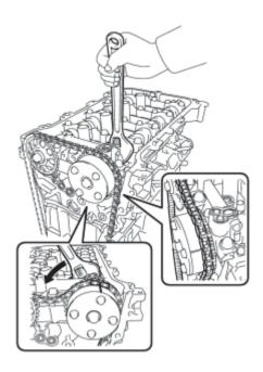
(b) With the chain loosened, release the chain from the camshaft timing gear and place it on the camshaft timing gear.
