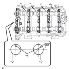
(b) Make sure of the marks and numbers on the camshaft bearing caps and place them in each proper position and direction.
