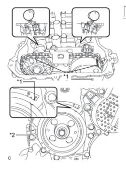
(b) Check that timing marks on both the camshaft timing sprocket and camshaft timing gear are facing upward as shown in the illustration.
