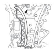
(a) Install the chain tensioner slipper to the cylinder block.
