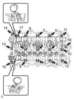
(c) Set the camshaft and No. 2 camshaft as shown in the illustration.
