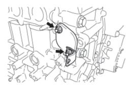
(a) Remove the 2 nuts, bracket, chain tensioner and gasket.
