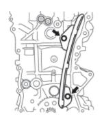
(a) Install the chain vibration damper with the 2 bolts.
