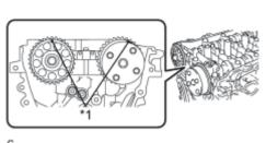
(c) Check that the timing marks on the camshaft timing gear and camshaft timing sprocket are aligned as shown in the illustration.
