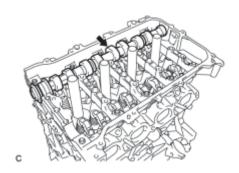
(a) Remove the No. 2 camshaft.
