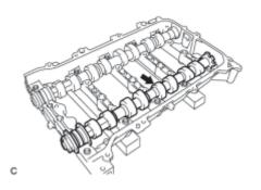
(c) Install the camshaft to the camshaft housing.
