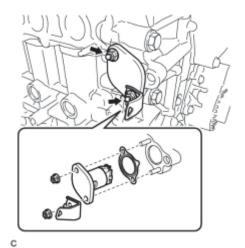
(b) Install a new gasket, the bracket and chain tensioner with the 2 nuts.
