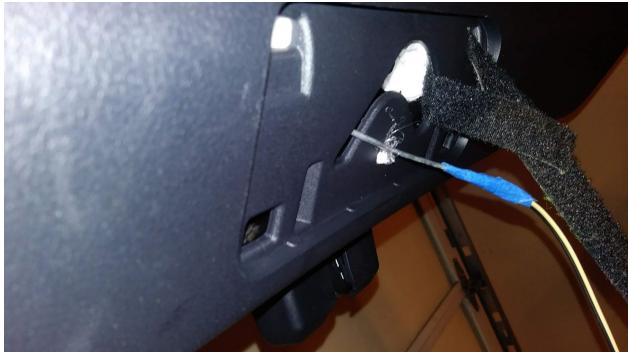
Tuck and run the wire inside the hollow space in both panel 1 & 2.
