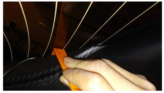
Now you need to open one more panel, that is on the top part inside the trunk door with 5 pins. Use both hands to pull from one end with some force, one pin at a time:
