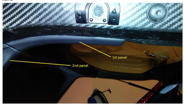
Insert some flat tool to pop 1st panel open slightly, you can see there is a hock anchoring:
