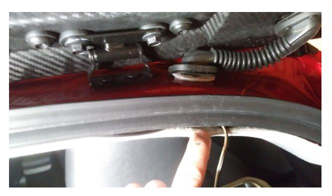
Pop open the cargo light module by inserting flat tool on the left side of it
