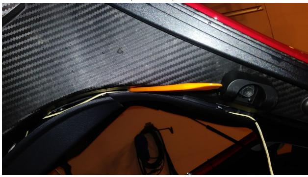
The wire should end up coming out from the top part of panel 1, we will hide the wire in between the glass and carbon fiber frame
