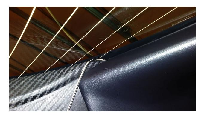
Continue to push the wire along the edge of the glass till you reach the top of the glass. The wire should not be visible from outside. Make sure you just use plastic tools to avoid damaging the heating wires.
