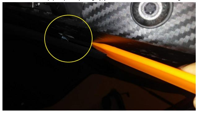
The 2nd panel can be opened partially to run the wires. Insert flat tool to expand the gap, the pull with some force to unlock one of the blue pin:
