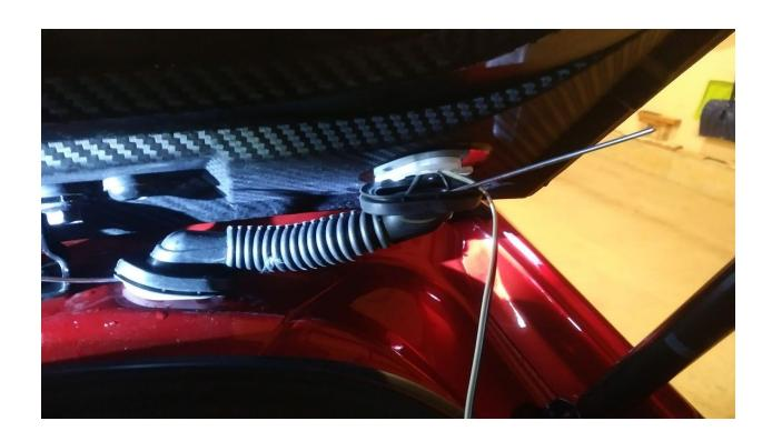
Remove the pin from the passenger roof near the edge of the trunk, so the we can get the wire out from the conduit to the cargo area
