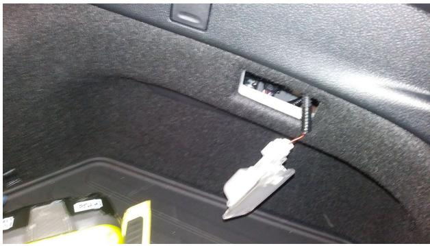
Pull the big rubber to expose the gap between the metal frame and interior cloth like material, continue to run the wire along the gap. Be Careful of the sticky black material, avoid touching them. Then fish the wire from that gap to the cargo light module opening. Connect the wire to your new LED light and tap the other end to the light module. You might want to disconnect the 12V battery first to avoid burning the fuse just in case if you shorted the circuit.
