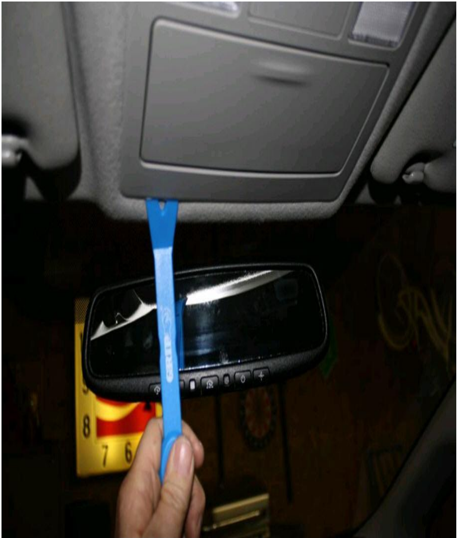
Locate push in points and pry downward.
