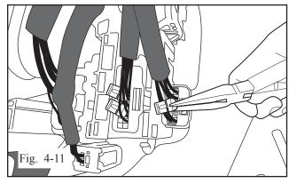
(1) Attach a BLUE T-tap connector to WHITE w/ BLACK TRACE wire (pin #2) with needle-nose pliers. (Fig 4-11)
