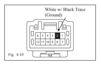
(k) Locate the WHITE w/ BLACK TRACE wire (pin #2) on the OL2 12 pin connector. (Fig. 4-10)
