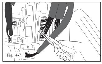
(h) Attach a RED T-tap connector to BLUE wire (pin #18) with needle-nose pliers. (Fig 4-7)
