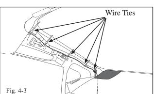
(d) Route the harness down the a-pillar, and secure to the OEM harness with (5) five wire ties. (Fig. 4-3)
