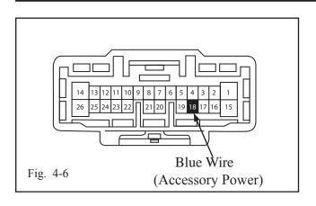
(g) Locate the BLUE wire (pin #18) on the OL1 26 pin connector. (Fig. 4-6)
