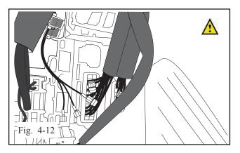
(m) Plug the BLACK w/ WHITE TRACE wire spade end of the EC mirror harness into T-tap connector on BLUE (pin #18) wire. (Fig. 4-12)
