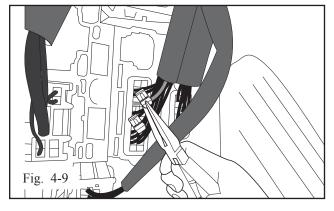
(j) Attach a RED T-tap connector to RED wire (pin #22) with needle-nose pliers. (Fig 4-9)
