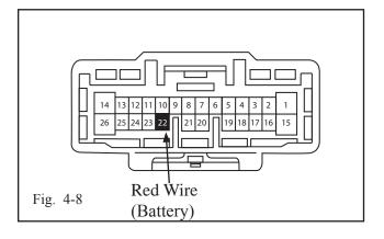
(i) Locate the RED wire (pin #22) on the OL1 26 pin connector. (Fig. 4-8)
