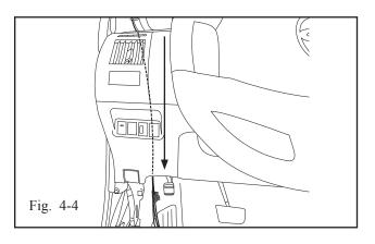
(e) Route the harness from the bottom of the a-pillar through the opening on the back of the dash, and into the driver side footwell. (Fig 4-4)
