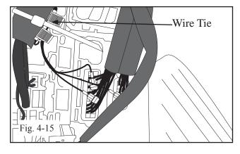
(p) Bundle any excess wire and secure it to the OE harness with one (1) wire tie as shown. (Fig. 4-15)
