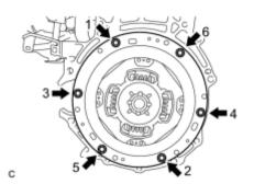
(c) In several steps, uniformly install and tighten the 6 bolts in the sequence shown in the illustration.
