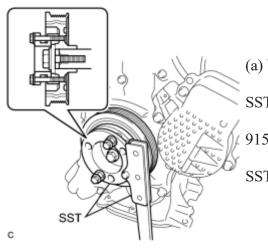
(a) Using SST, hold the crankshaft damper.
