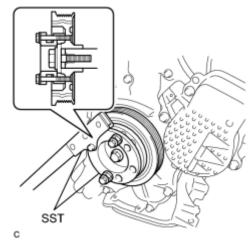
(a) Using SST, hold the crankshaft.
