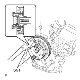
(b) Install the transmission input damper.
