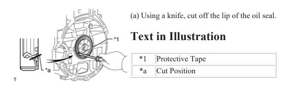
(b) Using a screwdriver with its tip wrapped with tape, pry out the oil seal.
