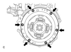
(b) Remove the 6 bolts and transmission input damper assembly from the flywheel sub-assembly.
