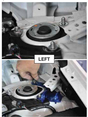
7.) Install the main bar with the washers and crush washer in this order. Hand tighten both ends, then torque down with a 17mm wrench and hex allen head driver.
