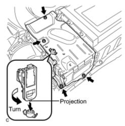
(a) Using the service plug grip, remove the battery cover lock striker.
