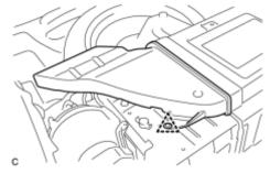
(a) Remove the clip and No. 1 hybrid battery exhaust duct.
