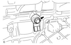
(b) Remove the bolt and remove the knock sensor.
