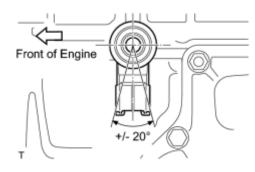
(a) Install the knock sensor with the bolt as shown in the illustration.
