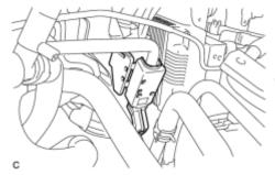
(b) Engage the lock claw to install the No. 1 fuel pipe clamp.
