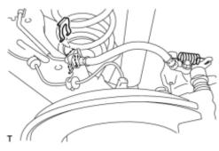
(b) Connect the rear flexible hose LH to the rear axle beam assembly with a new clip.
