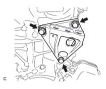
(g) Temporarily tighten the engine mounting bracket RH with the 3 bolts.
