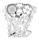
(c) Apply seal packing as shown in the illustration.
