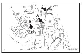
(2) Install the heater water pump with the 2 bolts. **NOTICE:**
