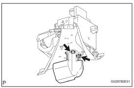
(i) Remove the brake actuator.
