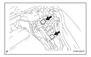
(1) With the power switch OFF to prohibit brake control, remove the No. 1 and No. 2 motor relays.
