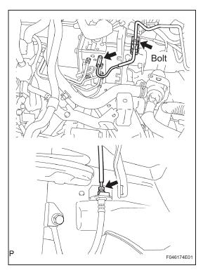
(3) Using SST, disconnect the No. 5 front brake tube from the brake actuator and front brake flexible hose.
