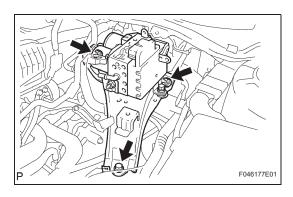
(10) Remove the bolt, 2 nuts and brake actuator with gusset.
