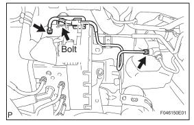
(2) Using SST, install the 4 brake tubes to the brake stroke simulator cylinder and brake actuator.
