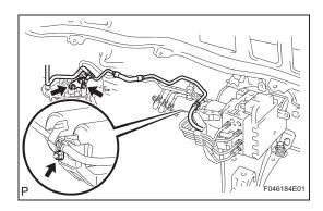
(7) Remove the 3 nuts and brake actuator tubes from the brake stroke simulator cylinder and brake actuator.
