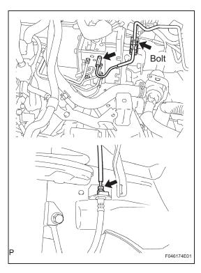
(8) Using SST, connect the No. 5 front brake tube.
