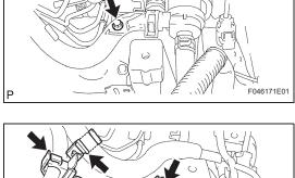
(3) Remove the 2 clamps, bolt and heater hose bracket from the gusset.
