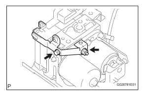
(2) Remove the bolt, nut and bracket from the brake actuator.
