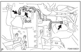
(5) Using SST, disconnect the No. 1 front brake tube.
