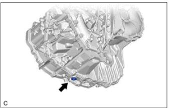
(d) Using a 10 mm hexagon socket wrench, temporarily install the drain plug and gasket to the hybrid vehicle transaxle assembly. [#4]
