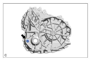
(c) Using a 10 mm hexagon socket wrench, remove the drain plug and gasket from the hybrid vehicle transaxle assembly and drain the hybrid transaxle fluid. [#3]
