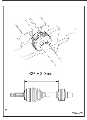
(a) Install the drive shaft damper to the outboard joint LH.
