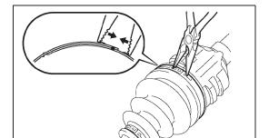
(b) When using a hook type:Using needle-nose pliers, unhook and remove the No. 2 inboard joint boot clamp.
