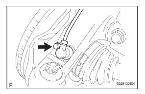
(b) Remove the bolt and front speed sensor from the steering knuckle.
