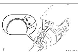
(b) When using a hook type: Using needle-nose pliers, unhook and remove the inboard joint boot clamp.
