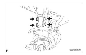
(c) Remove the 2 bolts and 2 nuts, and remove the front axle from the front shock absorber.
