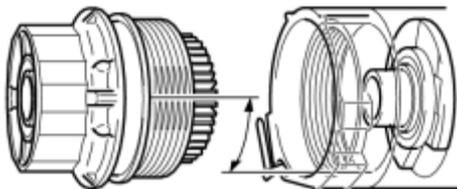
(e) Reapply a small amount of engine oil to the O-ring of the oil filter cap assembly. Align the cutout in the oil filter cap threads 90° to the grooves in the oil filter bracket and temporarily tighten the cap.
