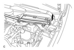
(c) Remove the center cowl top ventilator cover.
