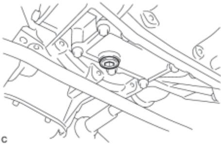
(b) Using a hexagon wrench (10 mm), remove the drain plug indicated in the illustration and drain the coolant.
