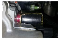
Guide the Red Bullet gently until it mates with the engine block.
