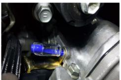
Rotate the body so that the securing tab on the Red Bullet aligns with the correct area on the engine.
