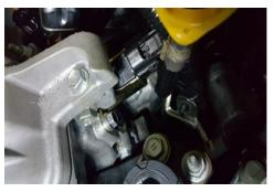
Tighten it with 10mm wrench to snug. There is no need to over tighten or torque down the bolt. Applying equivalent force required to loosen it in the beginning when extracting the OEM solenoid will suffice. Reconnect the signal plug.
