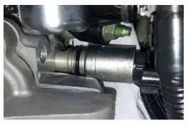
Once you free the part from the O-Ring groove, gently slide the solenoid outwards and clear it from the port. Store it away. There will be some oil coming out from the extraction process, which is totally normal and the quantity is very insignificant. You may check your oil level if you wish before and after the process.
