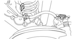
(b) Connect the rear flexible hose LH to the rear axle beam assembly with a new clip.
