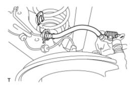
(b) Remove the clip and separate the rear flexible hose LH.
