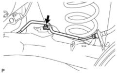
(a) Install the rear No. 4 brake tube to the rear axle beam assembly with the nut.
