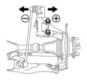
(e) Fully push or pull the front axle hub in the direction of the required adjustment. (Step B)
