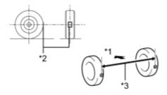
(d) Put tread center marks on the rearmost points of the rear wheels and measure the distance between the marks (dimension B).
