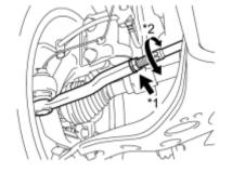
(c) Loosen the tie rod end lock nuts.
