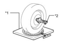
(a) Install a camber-caster-kingpin gauge and place the front wheels on the center of a wheel alignment tester.
