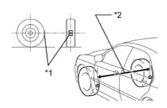
(d) Put tread center marks on the rearmost points of the front wheels and measure the distance between the marks (dimension B).
