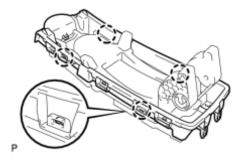
(a) Disengage the 4 claws and remove the inner console compartment door.
