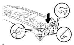
(a) Engage the 2 claws and 5 guides to install the rear console compartment door box cover as shown in the illustration.
