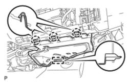
(b) Engage the guide and 3 claws to install the No. 2 instrument panel under cover sub-assembly.
