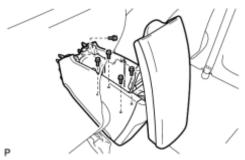
(c) Install the rear console box assembly with the 5 bolts.
