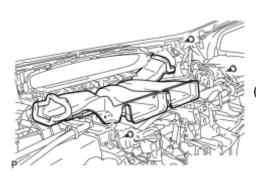
(a) Install the No. 1 heater to register duct with the 3 clips.
