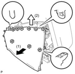
(b) Pull the No. 2 box side panel in the direction indicated by the arrow to disengage the 9 claws and guide, and remove the No. 2 box side panel.
