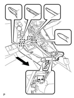
(b) While pushing the parts shown in the illustration inward, pull the console box assembly in the direction indicated by the arrow to disengage the 2 claws and 4 guides.
