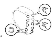
(a) Engage the 10 claws to install the console rear end panel.
