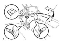
(a) Using a moulding remover, disengage the 3 claws to remove the upper console panel as shown in the illustration.
