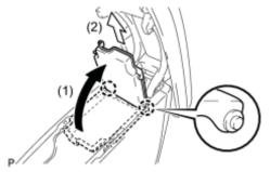
(a) Disengage the 2 claws and remove the console box pocket as shown in the illustration.
