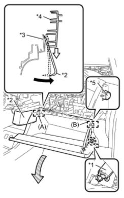
(a) Disengage the claw and release the glove compartment door stopper.
