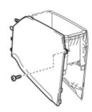
(b) Install the No. 2 box side panel with the screw.
