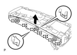
(a) Pull the No. 2 console compartment door insert in the direction indicated by the arrow to disengage the 3 claws and 7 guides, and remove the No. 2 console compartment door insert.
