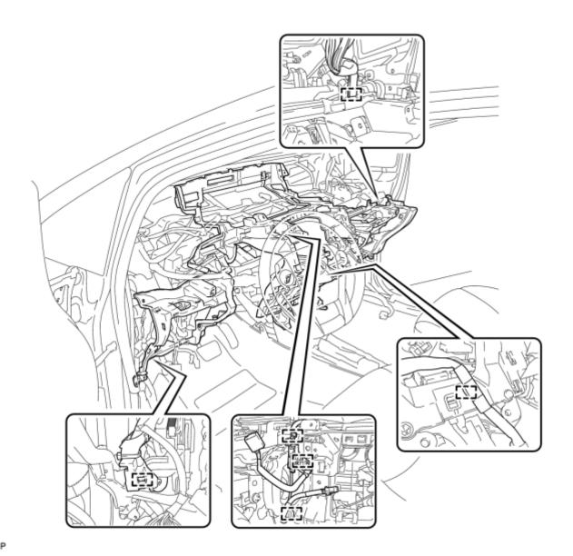
(b) Remove the 4 bolts <B>, 11 bolts <C>, screw <D> and lower instrument panel sub-assembly.
