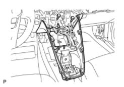
(c) Install the upper instrument panel finish panel assembly with the 2 bolts <A>.
