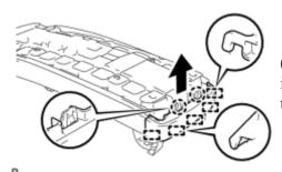
(c) Pull the rear console compartment door box cover in the direction indicated by the arrow to disengage the 2 claws and 5 guides, and remove the rear console compartment door box cover.
