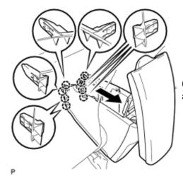
(b) Pull the rear console box assembly in the direction indicated by the arrow to disengage the 8 claws.
