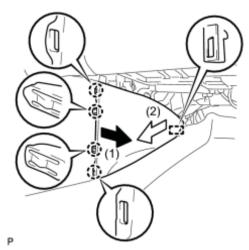
(a) Pull the front No. 2 console box insert in the direction indicated by the arrow to disengage the 4 claws and guide, and remove the front No. 2 console box insert.
