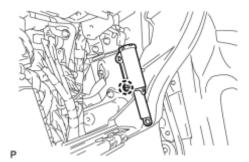
(a) Disengage the claw to remove the glove compartment door stopper sub-assembly.
