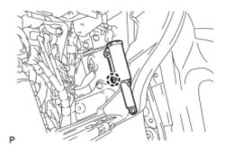
(a) Engage the claw to install the glove compartment door stopper sub-assembly.
