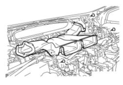
(a) Remove the 3 clips and the No. 1 heater to register duct.
