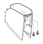
(a) Install the rear console compartment door sub-assembly with the 2 screws.
