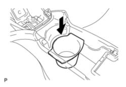
(a) Install the rear console box pocket as shown in the illustration.
