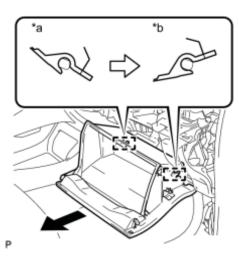
(d) Open the glove compartment door assembly to approximately 55° from its closed position. Pull it horizontally in the direction indicated by the arrow to disengage the 2 hinges and remove the glove compartment door assembly.
