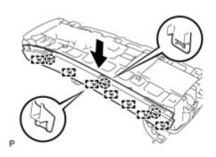
(a) Engage the 3 claws and 7 guides to install the No. 2 console compartment door insert as shown in the illustration.
