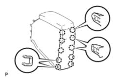
(a) Disengage the 10 claws to remove the console rear end panel.
