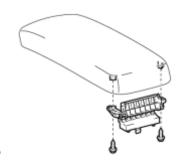
(a) Remove the 2 screws and the console compartment door hinge sub-assembly.
