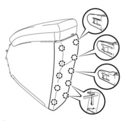
(a) Engage the 10 claws to install the console rear end panel.
