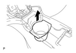
(a) Remove the rear console box pocket.
