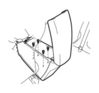
(b) Install the rear console box assembly with the 4 bolts.
