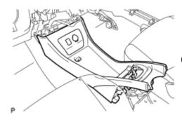
(a) Temporarily install the console box assembly.
