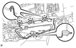
(a) Disengage the 3 claws and guide.
