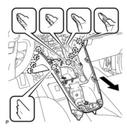
(c) Pull the upper instrument panel finish panel assembly in the direction indicated by the arrow to disengage the 9 claws and remove the upper instrument panel finish panel assembly.
