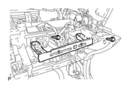
(a) Install the instrument panel safety pad plate sub-assembly with the 2 bolts <B>.
