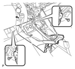
(c) Install the console box assembly with the bolt <B> and 2 clips.
