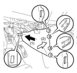
(a) Engage the guide and 4 claws to install the front No. 1 console box insert as shown in the illustration.
