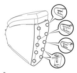
(a) Disengage the 10 claws to remove the console rear end panel.
