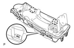
(b) Engage the 4 claws to install the inner console compartment door.
