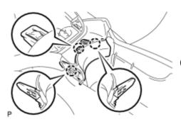
(a) Engage the 3 claws to install the upper console panel.
