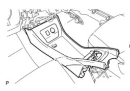
(a) Remove the console box assembly.
