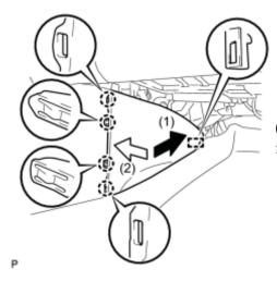
(a) Engage the guide and 4 claws to install the front No. 2 console box insert as shown in the illustration.
