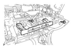
(a) Remove the 2 bolts <B> and instrument panel safety pad plate subassembly.
