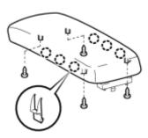
(b) Install the outer console compartment door with the 4 screws.
