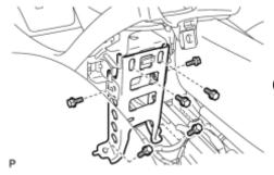
(a) Remove the 6 bolts <B> and No. 2 console box mounting bracket.
