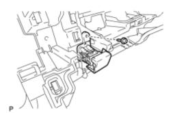
(a) Remove the screw <D> and glove compartment door lock assembly.
