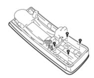
(c) Install the outer console compartment door with the 4 screws.
