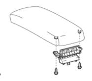
(a) Install the console compartment door hinge sub-assembly with the 2 screws.
