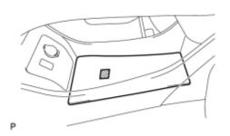
(a) Disengage the fastener and remove the box bottom mat.
