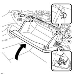
(b) Slightly bend the stoppers (A) and (B) in the directions indicated by the arrows in the illustration and engage the stoppers to install the glove compartment door assembly.
