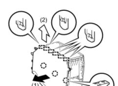
(b) Disengage the 3 claws and 6 guides and remove the No. 2 box side panel.
