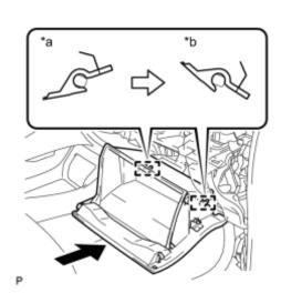
(a) With the glove compartment door assembly opened approximately 55° from its closed position, engage the 2 hinges horizontally.
